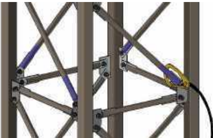
FIGURE 1 FIGURE 1 - LANYARD HOOK SAFE PLACEMENT (PURPLE SHADING)
